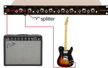
2. Lower the send level control and move the cable that feeds the amp to the send output instead. Now adjust the send control so you get the same amp level as you got when the amp was connected to the "Y" splitter.
