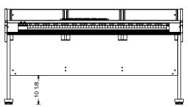
The "Controller" version of the Multi-Station is configured for the small footprint keyboards that are 10 1/2" deep (or less).
