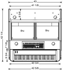
The "Controller" version of the Multi-Station is configured for the small footprint midi controllers that measure up to 10 1/2"deep (or less). This size keyboard allows the qwerty keyboard and mouse / trackball to be placed on the convenient shelf (A) located behind the keyboard.
