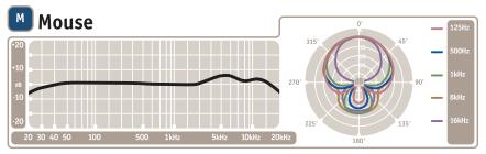
This frequency chart of the Mouse capsule is only a start. It gives the recordist a basis of the sound provided. How the microphone reacts in a particular application will differ greatly because of many variables. Room acoustics, distance from sound source (proximity), tuning of the instrument and microphone cabling are only a few of the interacting issues. For an artist or engineer, how the microphones are used creates the basis of the sound.
