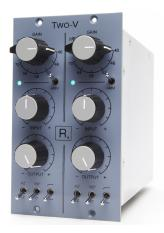
In addition to its unique gain structure this circuit also provides +48 volt phantom power, input impedance selection, polarity inversion and an extremely musical, broadly applicable hi-pass filter per channel. The Two-R rack unit further adds a true hi-impedance (2 M $\Omega$ ) 1/4" instrument input per channel.
