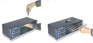
Two Phillips screws on the bottom of the Workhorse allow the slide-in tray to be taken out. To remove, turn the workhorse upside down and locate the two Phillips head screws on the bottom chassis. Remove the two screws and lift out the tray. Replacing the two screws back into the slide-in tray will help keep them handy if the tray is to be re-installed.
