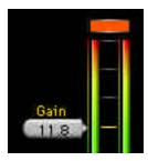
Just above the Input/Ouput meters is the indicator for the built-in limiter. The Renaissance Compressor has an L1-style limiter at the output stage, and works well in compression or expansion modes. Threshold and Output Ceiling is set to 0dBFS and it is activated only when the level would exceed 0dBFS. On activation, the limiter action is in addition to the compression, and the total actualy gain reduction is shown in the gain reduction meter.
