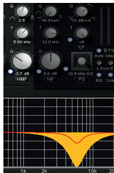
Auto listen "Q" with NEGATIVE gain [see the HMF band gain at (-3.7dB)]
