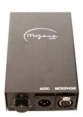
Cardioid: 12 o'clock position. Cardioid microphones pick up sound within 120 degrees of the direction they are facing. Useful for capturing one sound with a minimum of ambiance.
