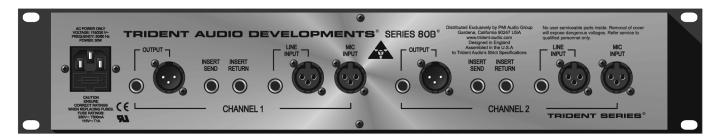
The rear panel of the unit provides both XLR and  $\frac{1}{4}$ " jack inputs for the line input and output of each channel while a separate XLR is provided for the microphone input. The insert sends and returns are balanced  $\frac{1}{4}$ " jacks. The XLR connectors use the standard industry convention of pin 1 ground, pin 2 positive and pin 3 negative. The jacks are tip-positive, ring-negative and sleeve ground. For unbalanced use, connect the ring to the sleeve.
