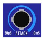
**ATTACK:** Sets the time it takes the compressor to react when levels exceed the set **THRESHOLD**
