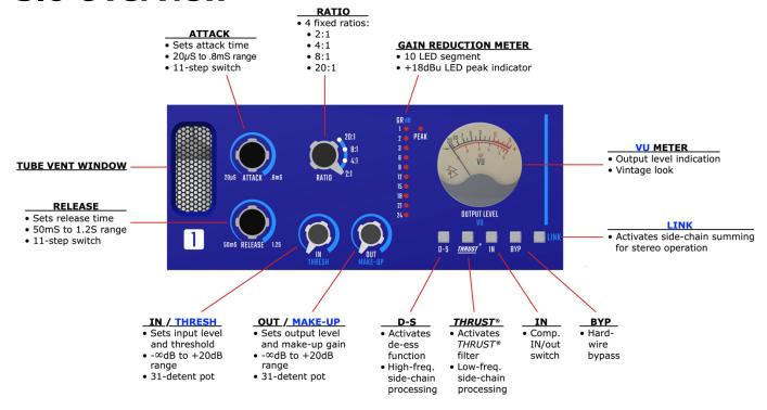
The T25 Tube Compressor provides a comprehensive suite of controls:
