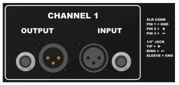
IMPORTANT NOTE: The XLR and ¼" INPUT connectors are wired together, so use only one INPUT connection a time.
