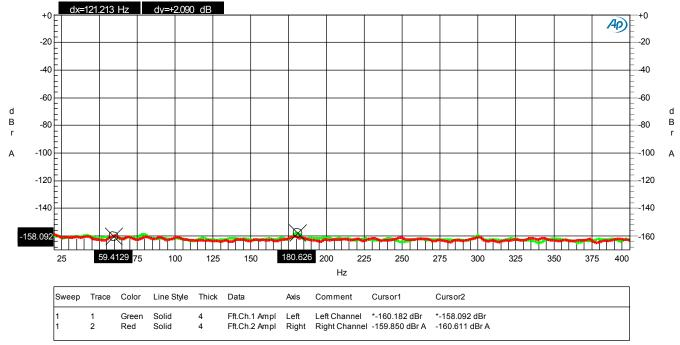
DAC3 - FFT Idle Channel Noise - Low Frequency.at27
