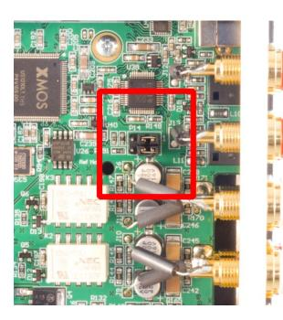
Figure 8 - Digital PASS-THROUGH Disabled (Factory Default)
