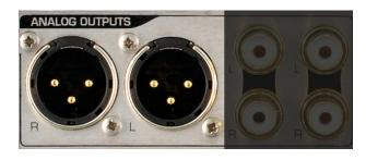
The Left and Right balanced outputs use Neutrik™ gold-pin male XLR jacks. The XLR shell and pin 1 (ground) are both directly bonded to the chassis to prevent currents in the internal ground system. This direct bonding also maximizes RF shielding.
