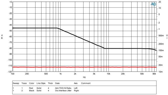
DAC3 - JITTER TOLERANCE.at27
