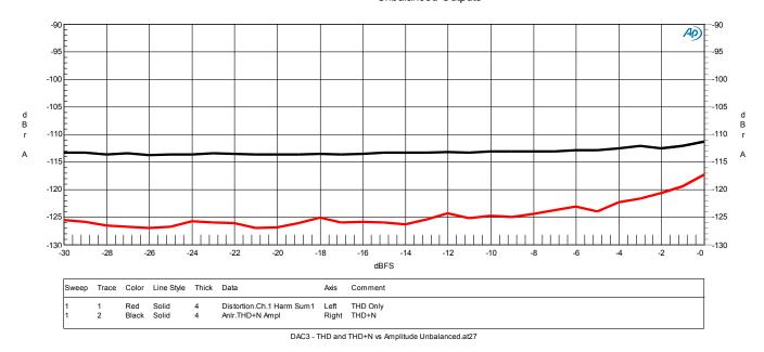
**Graph 8 - THD and THD+N vs. Amplitude (Unbalanced Outputs)**
