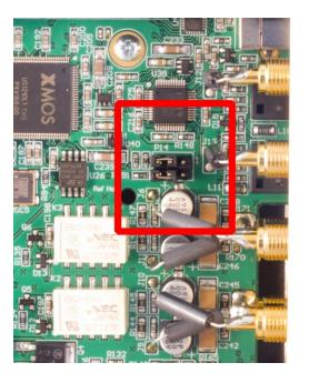
Figure 7 - Digital PASS-THROUGH Enabled
