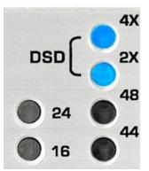
Two lights indicate the measured word length of the selected digital input.
