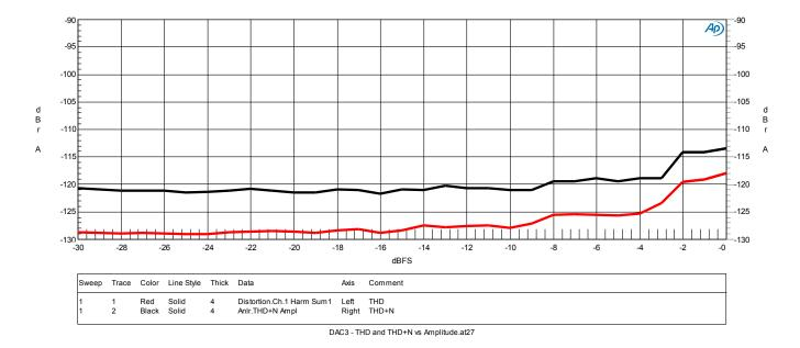
**Graph 7 - THD and THD+N vs. Amplitude (Balanced Outputs)**
