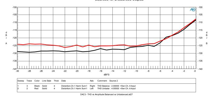
Graph 9 - THD vs. Amplitude - Balanced vs. Unbalanced Outputs
