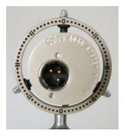
The 4050 microphones are attached to the shock mount via magnets enabling them to be swivelled through  $360^{\circ}$ . The unique shock mount has graduations allowing the microphones to be precisely positioned.
