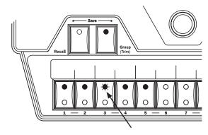
One channel in a Group is always available for editing, indicated by a flashing LED; press any other channel in the Group to change its pan or volume.
