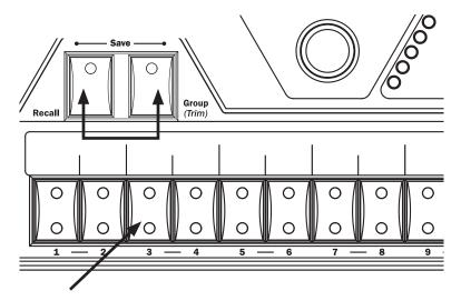
To save a Preset, hold Recall and Group simultaneously and then press a channel button.
