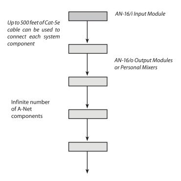
Your cable length performance will be affected by a number of factors including the quality of the cables used, and the number of devices such as cable couplers used or passive wall panel interconnections in use. Use Cat-5e cable for best performance wherever possible. Stranded or solid Cat-5e cable can be used.
