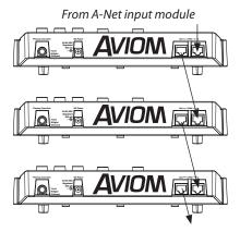
Connect A-Net Out to A-Net In to make a daisy chain.
