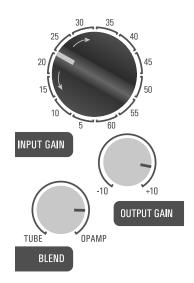
On vocals, try using the TUBE path for an intimate vocal, balance the INPUT GAIN and OUTPUT GAIN to accentuate a proximity effect on a condenser mic.
