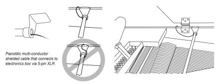
Figure 7. Positioning the PianoMic Cable
