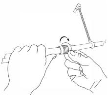
Figure 3. Loosening the Clutches
