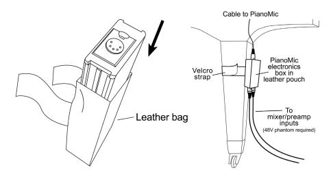
Figures 14. Placing the Electronics Box in the Pouch.
