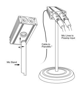
Figure 16. Mounting Electronics Box on Microphone Stand Adapter Bar
