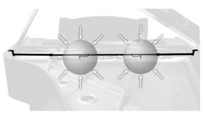
Figure 2. Random Incidence Microphones Inside a Piano
