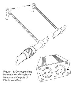
via a 5-pin XLR connector. The bottom of the electronics box has two XLR-3 connectors that will connect the microphone outputs to the preamp inputs of your mixer.
