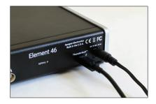
Connect the Power Supply to Element.
