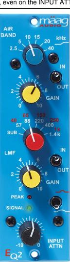
AIR BAND IN/OUT Engages and disengages the AIR BAND
