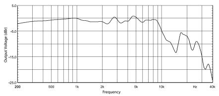
Displayed range from 200 Hz up due to measurement room size limitations 0 dBr = 2.8 mv / Pa
