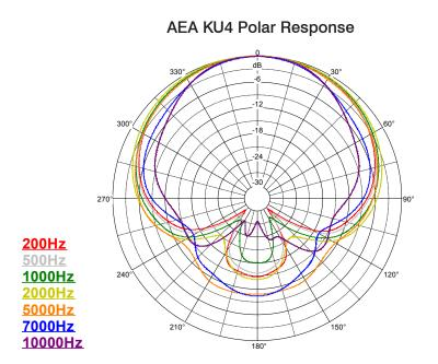
The reduced rear-lobe of the supercardioid pattern means that compared to a conventional bidirectional ribbon microphone, the KU4 will have less pickup of ambient noise or other sounds approaching from the rear. This makes it much easier to use in situations where isolation between instruments is important.
