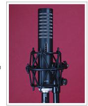
the mic's built-in wind-shielding is quite effective and does provide some extra peace of mind.
