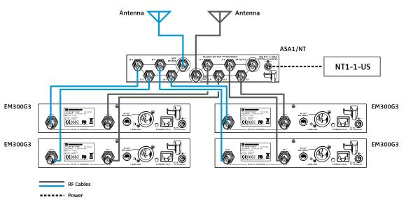
PRO TIP: DC Power for (EM) receivers is provided via the "A" Outputs
