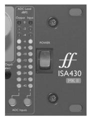
Two LED bargraph meters monitor the level being fed to the output (left meter) and input (right meter) of the unit.
