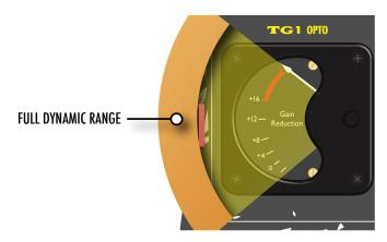
Without applying signal (or bypassed), adjust the 'HOLD' knob to place the meter's needle for the desired amount of compression (counterclockwise equals more compression).
