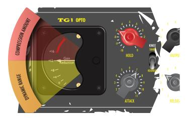
Without applying signal to the compressor (or bypassed), set the 'HOLD' knob fully clockwise (0), placing the meter's needle at the top of the scale range. This setting is equivalent to zero compression, i.e. full dynamic range.
