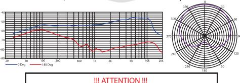
This is an END - FIRE microphone. Audio is acquired from the END of this microphone, NOT the side.
